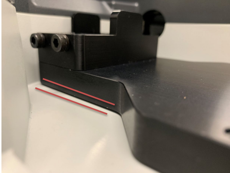
Figure 5: Baseplate installed flush with instrument body
